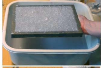
Sometimes the paper doesn't turn out right. In that case you can just turn the mold upside down and dip it in the water. The pulp will release from the mold easily.
